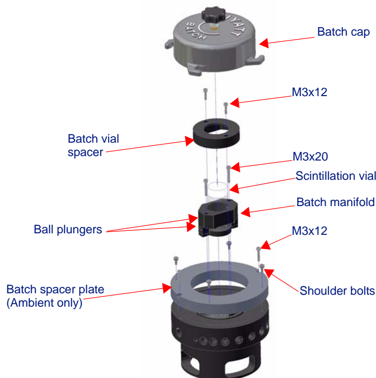
Figure 5-11: Flow-to-batch conversion kit, exploded
