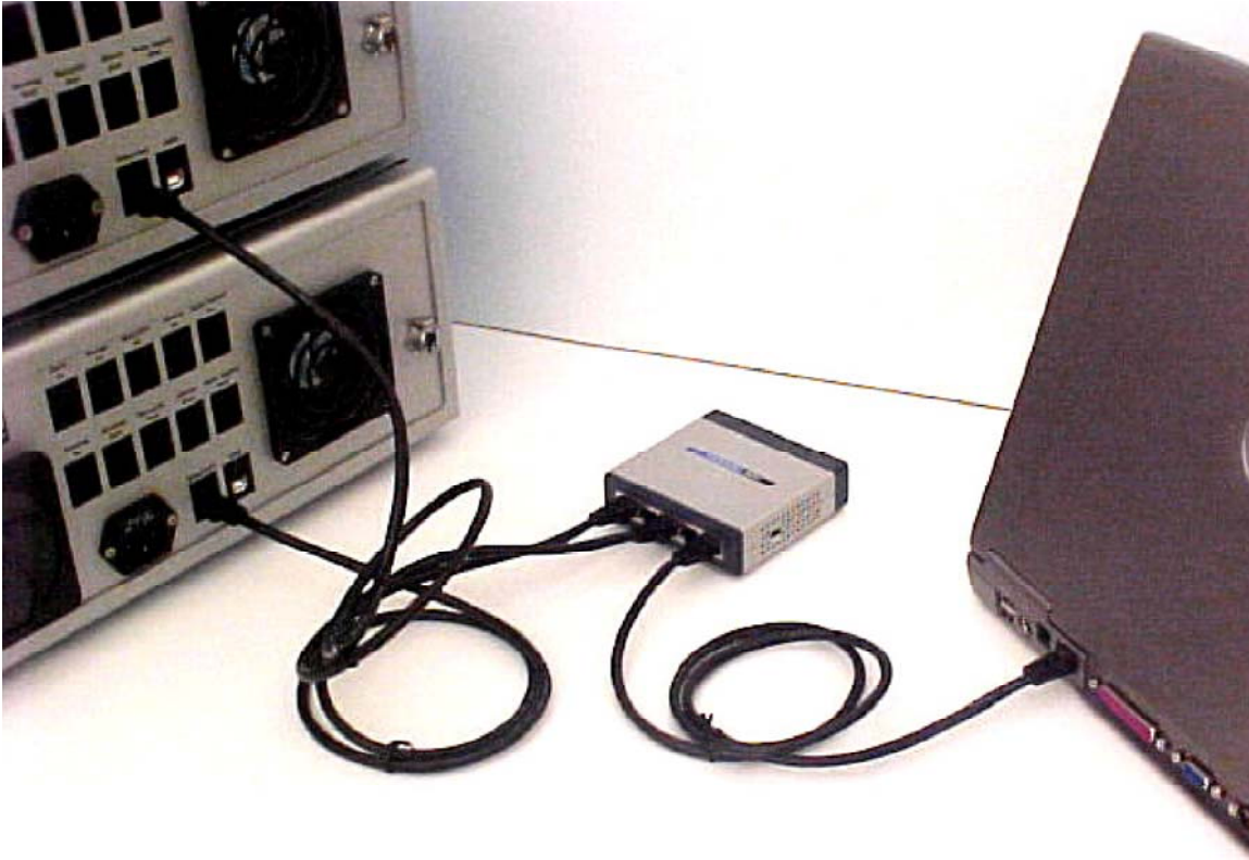
Figure D-17: Connecting multiple instruments to a computer not on the LAN using an Ethernet switch.
