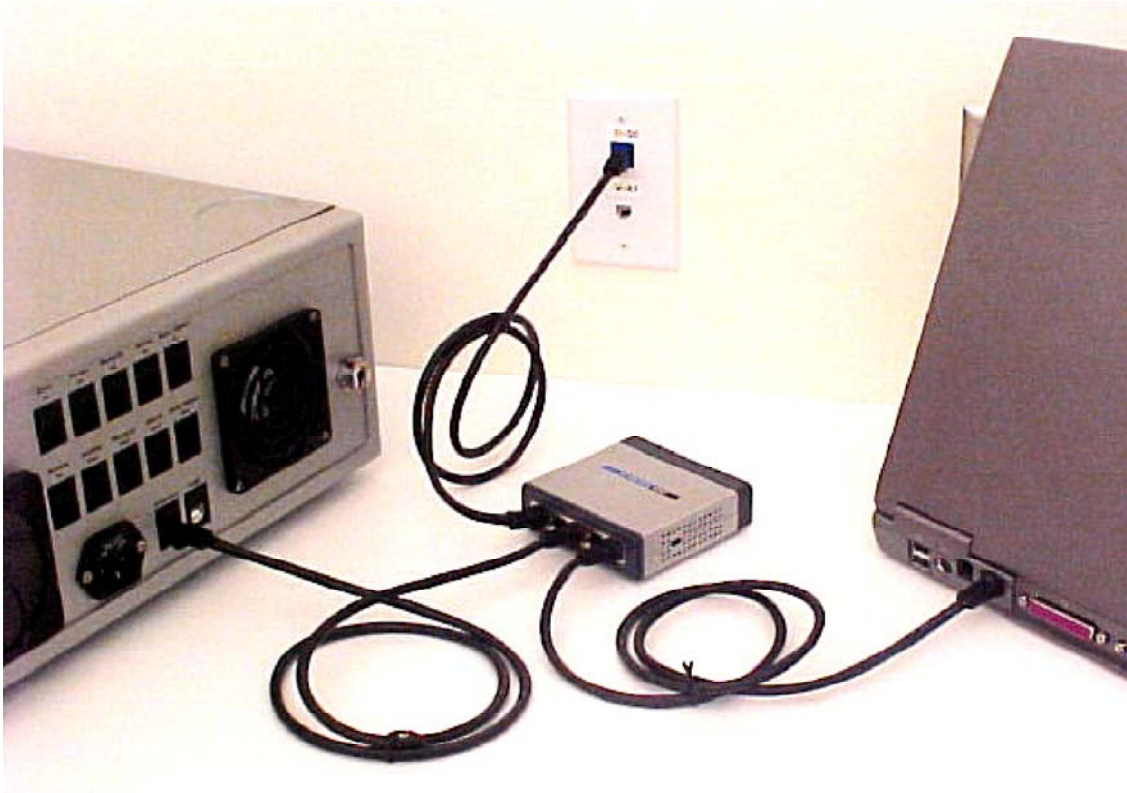
Figure H-9: One instrument and a computer can both be connected to the LAN using an Ethernet switch.
