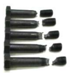
Fig. 2: Bolt Fractures (From Top) 0 Threads to 8 Threads
