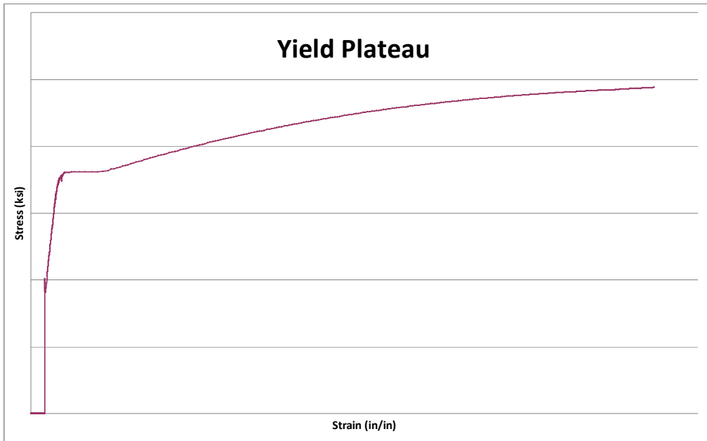
Fig. 2-2: Stress-Strain curve with apparent yield plateau
