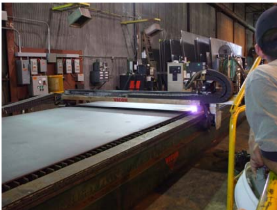
Figure 4. Flame Cutting Steel Piece
