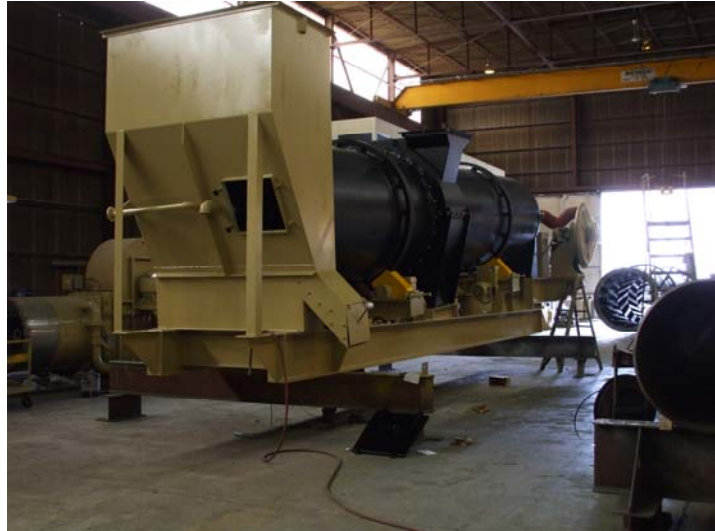
Figure 3. Completed Asphalt Mixer
