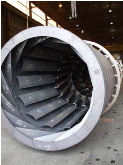
Figure 2. Inside of Asphalt Mixer
