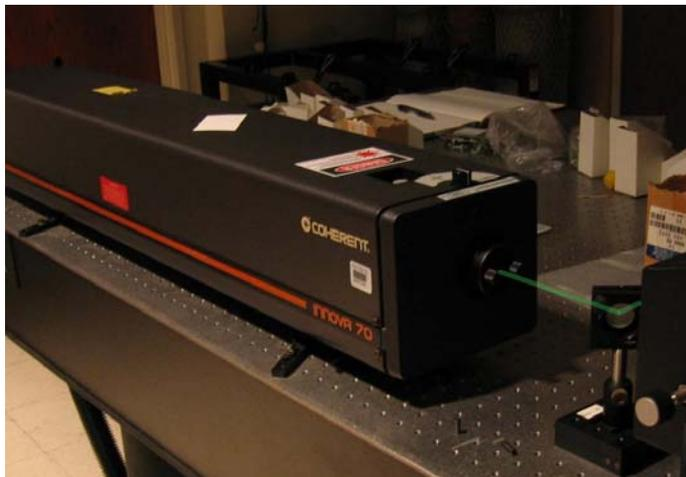
**Figure 5.** Ar ion laser, generating 514 nm light (green), 488 nm (blue) among other lines. This laser emits high levels of radiation. Use safety goggles.
