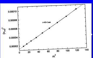
Squares of the positions of the intensity maxima versus squares of the Kiessig fringe order "m" is plotted
