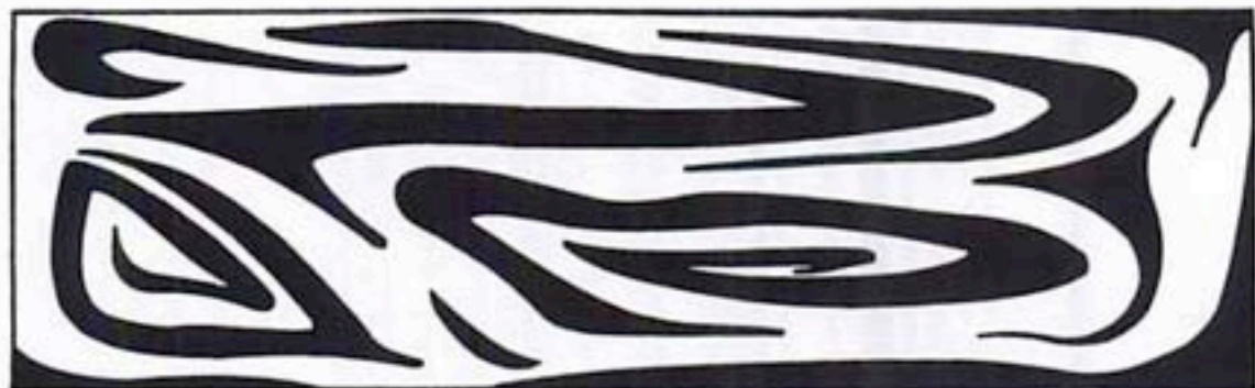
Figure 1 Mixture section similar to those observed in single-screw extruders.
