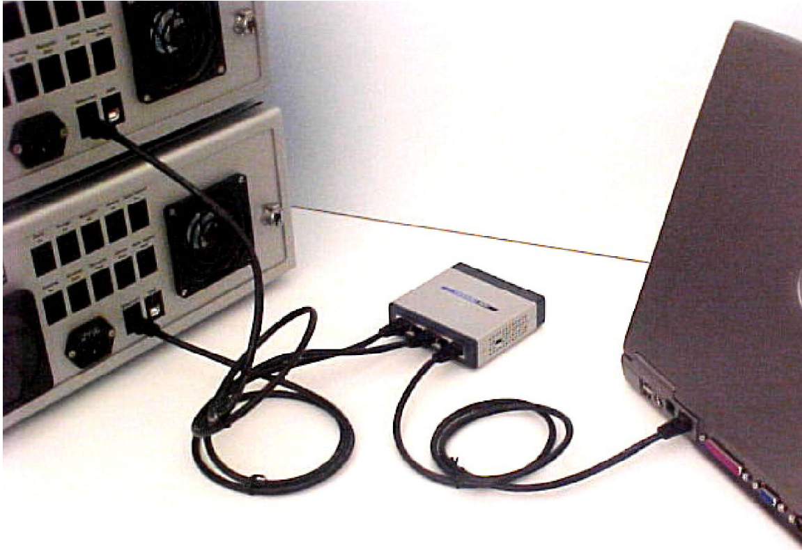
Figure H-17: Connecting multiple instruments to a computer not on the LAN using an Ethernet switch.
