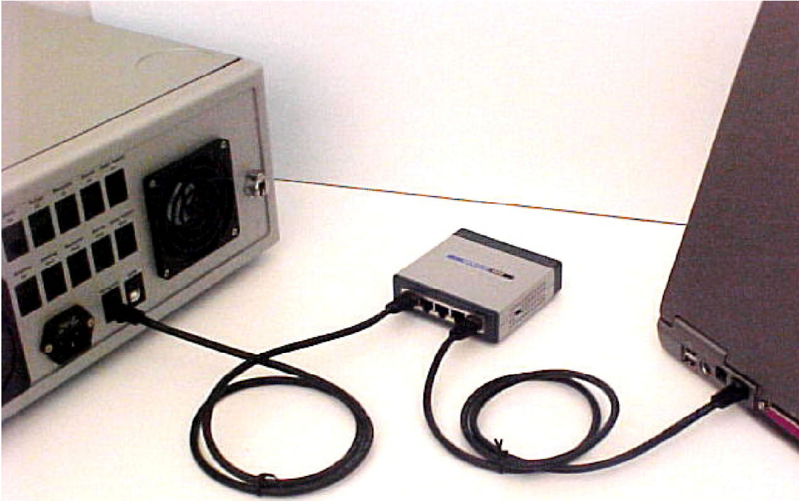
Figure H-16: Connecting one instrument to the computer using an Ethernet switch.
