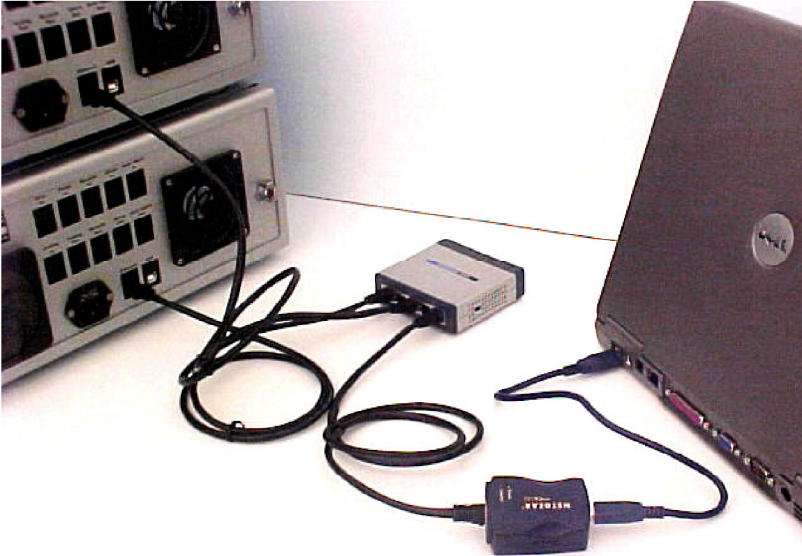
Figure H-14: Connecting two or more instruments to USB using an Ethernet switch and Ethernet to USB adapter.
