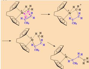
For polypropylene this switching of the reaction orientation leads to isotactic polymer,
