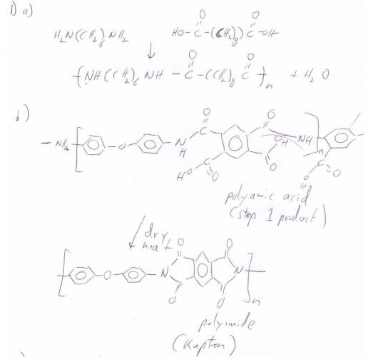
c) Both involve condensation reaction of a diamide and a dicarboxylic acid or an anhydride. For the polyimide the reaction occurs twice.
