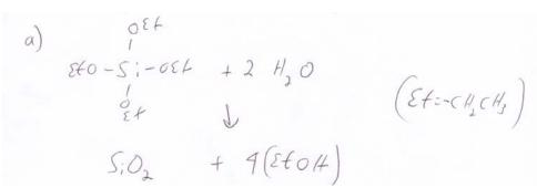
b) Acid or base can be used as a catalyst. The structure of the product is different for acid and base.
