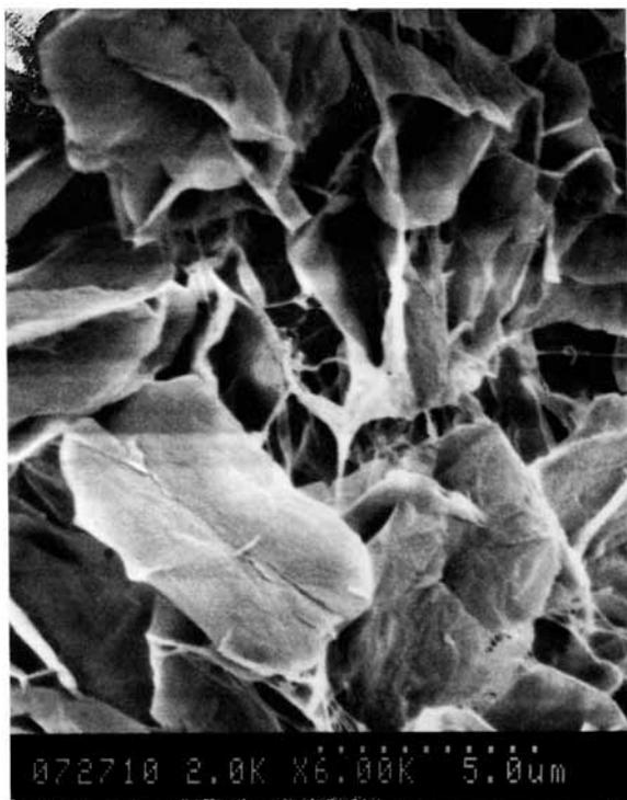
**Figure 11.** Disordered lamellae. NBS 1484, 5% w/w, run S-11.
