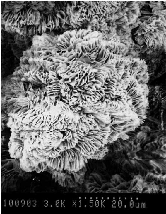
**Figure 7.** Coiled, sphere-like structures. HDPE 1 at 19.8% w/w, run S-36.
