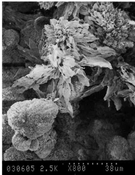
**Figure 18.** Morphologies believed associated with both the dilute (vapor) and the concentrated (liquid) phases after phase splitting during crystallization of run S-49.
