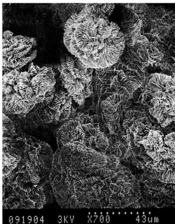
**Figure 6.** Coiled, sphere-like structures. HDPE 1 at 19.8% w/w, run S-36.
