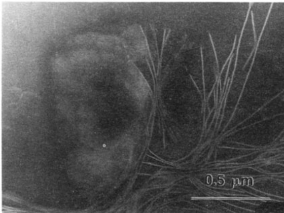
Figure 18. Lamellar growth in cis -polyisoprene in regime I showing the characteristic leaf-shaped profiles of the lamellae in the 'turned over' orientation.
