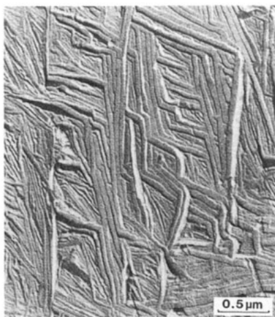
Figure 19. Transmission electron micrograph of a shadowed carbon replica of permanganically etched linear polyethylene showing ridged crystals. The specimen ( M_w = 37\,000 , M_n = 29\,000 ) had been crystallised at 130 °C for 7.5 days followed by 30 min at 125 °C prior to a cold-water quench. (Bassett and Hodge, unpublished work. Photograph supplied by D C Bassett.)
