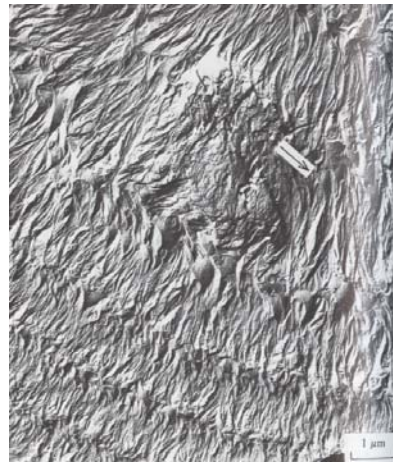
Fig. 3.8. Six sectors in a truncated polyethylene lamella revealed in situ from Bassett, Frank & Keller, 1979.
