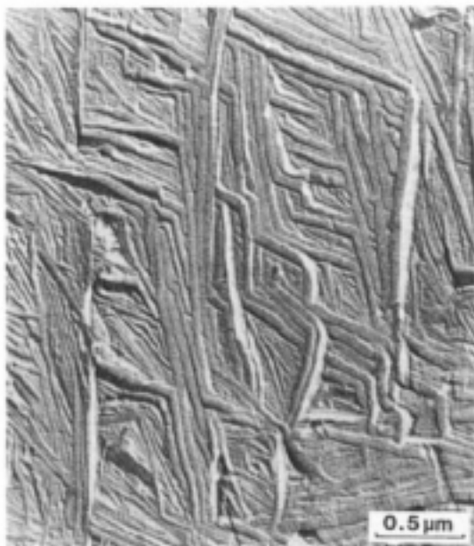
Figure 19. Transmission electron micrograph of a shadowed carbon replica of permanganically etched linear polyethylene showing ridged crystals. The specimen ( M_w = 37\,000 , M_n = 29\,000 ) had been crystallised at 130\text{ }^\circ\text{C} for 7.5 days followed by 30 min at 125\text{ }^\circ\text{C} prior to a cold-water quench. (Bassett and Hodge, unpublished work. Photograph supplied by D C Bassett.)
