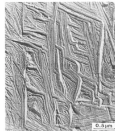
Figure 19. Transmission electron micrograph of a shadowed carbon replica of permanganically etched linear polyethylene showing ridged crystals. The specimen ( M_w = 37\ 000 , M_n = 29\ 000 ) had been crystallised at 130^{\circ}\text{C} for 7.5 days followed by 30 min at 125^{\circ}\text{C} prior to a cold-water quench. (Bassett and Hodge, unpublished work. Photograph supplied by D C Bassett.)
