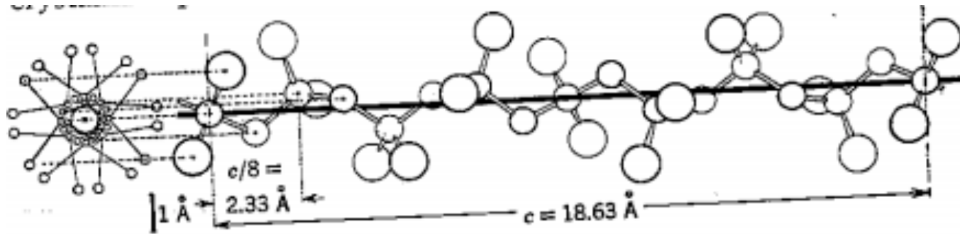
Figure 6-8 The 8/5 helix of the polyisobutene molecule. Small circles = CH 2 ; large circles = CH 3 . (Liquori [25].)
