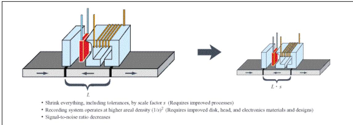
**Figure 3** Basic scaling for magnetic recording [4]
