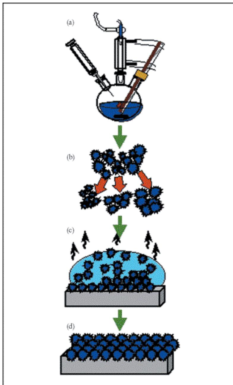
**Figure 6** Schematic representation of the synthetic procedures to (a) synthesize nanocrystal samples by high-temperature solution-phase routes, (b) narrow the nanocrystal sample size distribution by size-selective precipitation, (c) deposit NC dispersions that self-assemble, and (d) form ordered superlattices [11]
