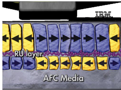
**Figure 4** Schematic illustration of AFC with single magnetic transition [8]
