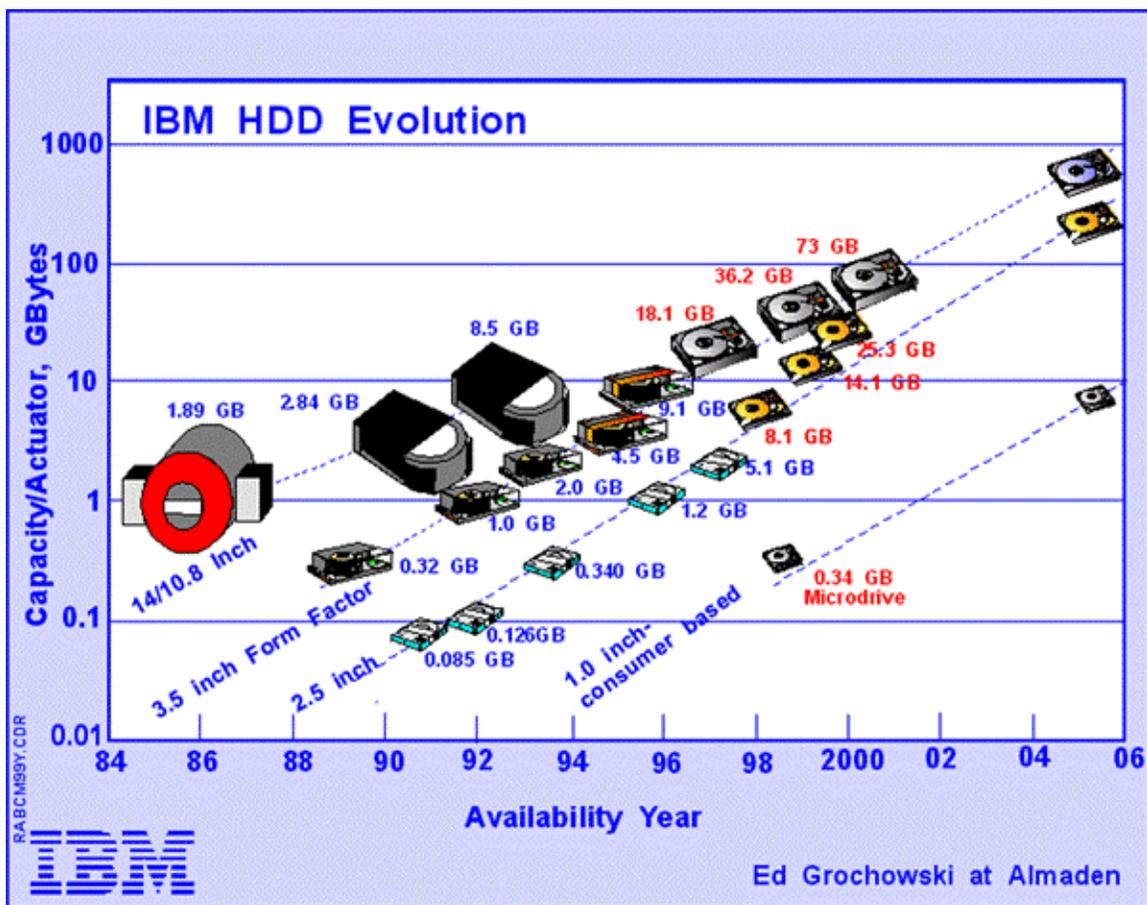
**Figure 2** Evolution of IBM hard disks over the past 15 years [3] Note the decreasing form factors from 14" to 1.0" as one moves from 1984 to the present.
