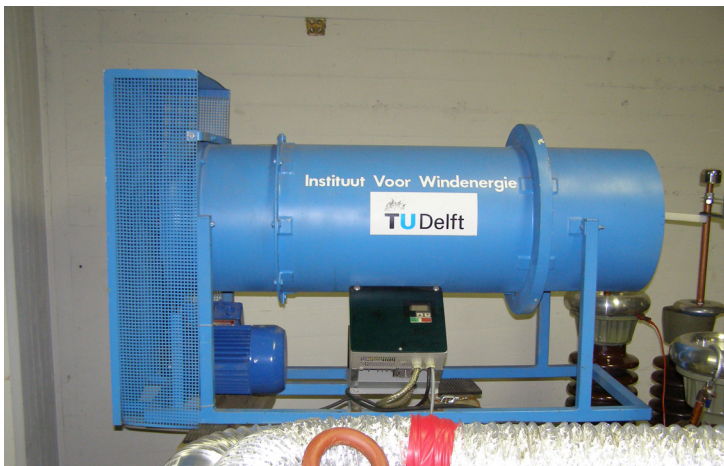
Figure 4.3. The wind generator which has been used to provide laminar air flow to move the charged droplets away from the charging system.
