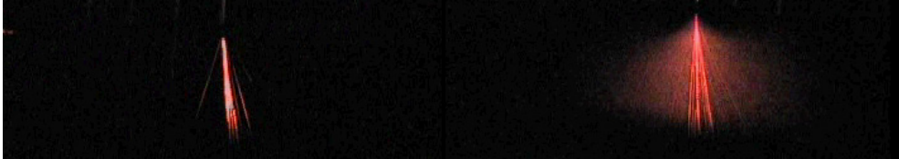
Figure 3.5. A photo of the spraying process using water/ethanol as the spraying liquid. Both a positive charging potential, on the left, and a negative charging potential, on the right, was used. The spray is illuminated with laser light. Note the presence of a fine mist on the right.
