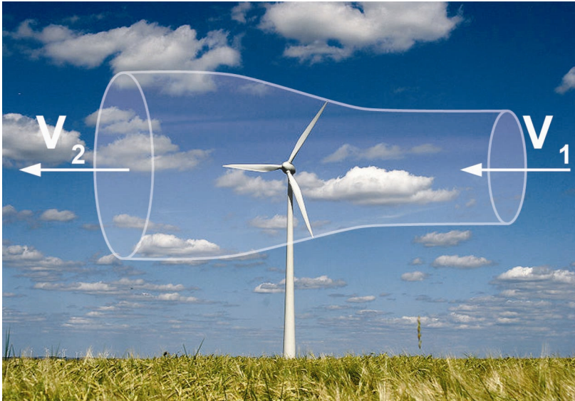
Figure 2.1. Illustration of the Betz limit. The wind speed behind the wind converter, v_2 , should ideally be \frac{1}{3} of the speed before it enters the converter, v_1 , while the speed just in front of the converter is \frac{2}{3} of the initial wind speed.
