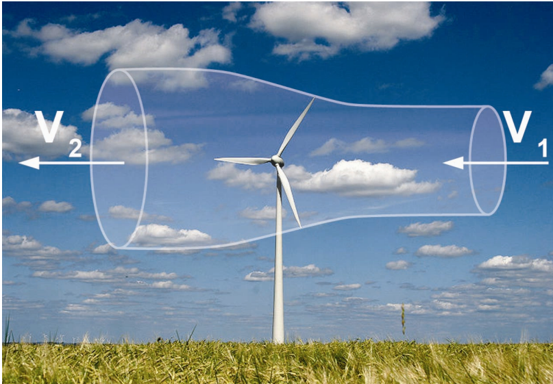
Figure A.1. Illustration of the Betz limit.
