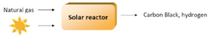
Figure 2 Hydrogen production by industry vs. via solar cracking
