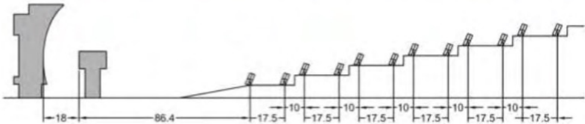
Elevation view of the Odeillo MWSF facility
