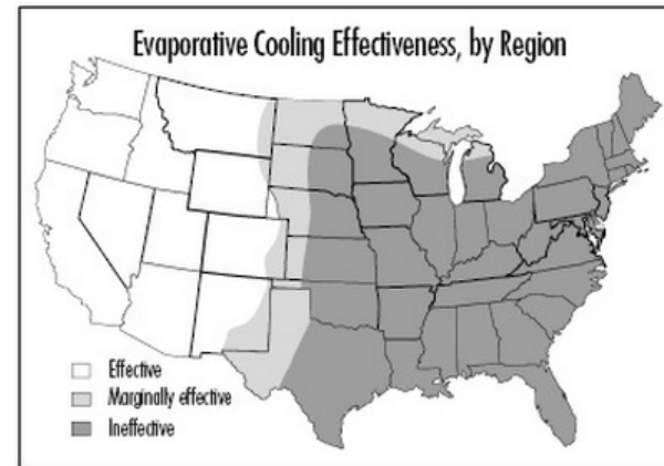
Figure 2. In areas of the United States where humidity tends to run high in the summertime, evaporative cooling is not the best way to stay cool; in the West, it's a very good choice.
