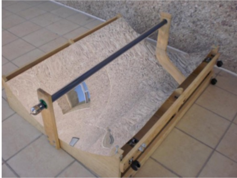
Figure 8 Picture of the prototype in its final version with the evacuated tube receiver.
