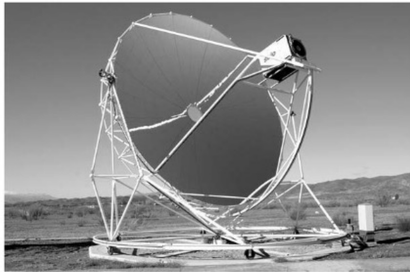
FIGURE 3.20 Parabolic dish collector. (a) Schematic diagram. (b) Photo of a Eurodish collector (from www.psa.es/webeng/instalaciones/discos.html ).
