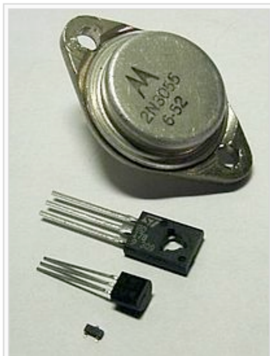
Assorted discrete transistors. Packages in order from top to bottom: TO-3, TO-126, TO-92, SOT-23
