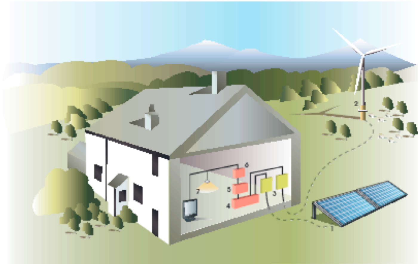
Figure 5.1 Remote and independent: a stand-alone system for a farmhouse.
