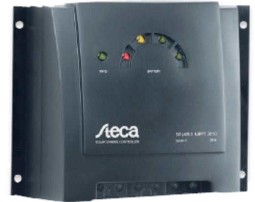
Figure 5.9 This MPPT controller can control a 12 or 24 V system with PV array power up to 500W p and MPP voltages up to 100V. With dimensions 19 × 15 × 7 cm, it weighs 900g (Steca Elektronik GmbH).
