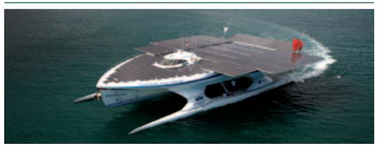
Photo 5.4 This 31-m demonstration boat is circumnavigating the globe, powered only by its PV panels
