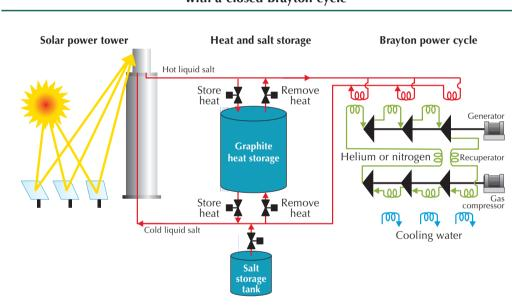
Figure 8.3 Scheme of fluoride-liquid salt solar tower associated with a closed Brayton cycle
