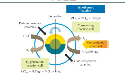
Figure 9.3 Two-step water splitting based on redox reactions generating H<sub>2</sub> from sun and water
