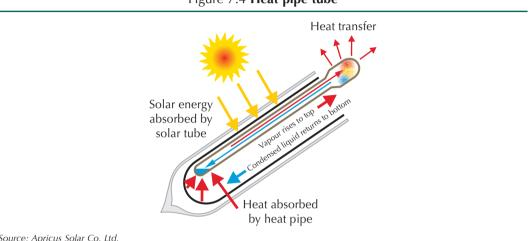
Figure 7.4 Heat pipe tube
