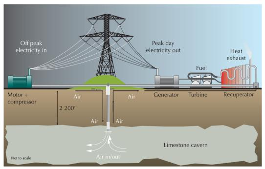
Figure 3.8 Compressed-air storage system
