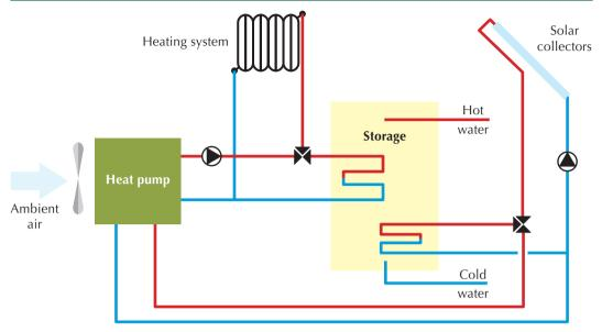
Figure 4.9 Combination of ASHP with solar collectors
