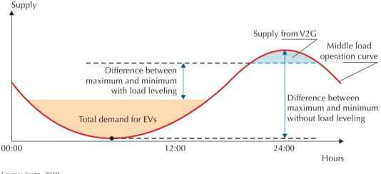
Figure 11.6 How EV and PHEV batteries can help level the load on the electric grids
