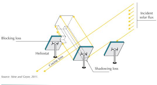
Figure 7.10 Blocking, shading and cosine losses in heliostat fields
