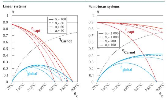
Figure 8.1 Efficiencies as a function of temperature for various concentration ratios
