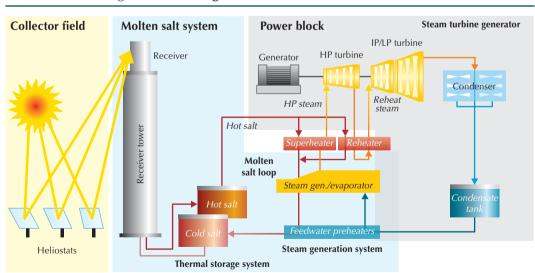
Figure 8.2 Working scheme of a molten-salt solar tower
