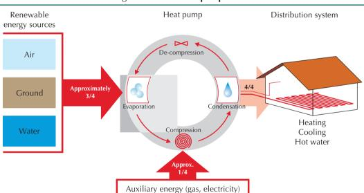
Figure 4.7 How heat pumps work
