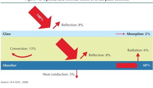
Figure 7.2 Optimal and thermal losses of a flat-plate collector
