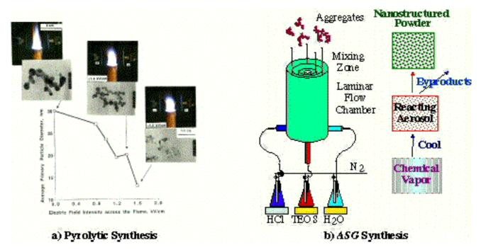
Two synthetic processes used at the University of Cincinnati for the synthesis of nano-aggregates for elastomer reinforcement.
