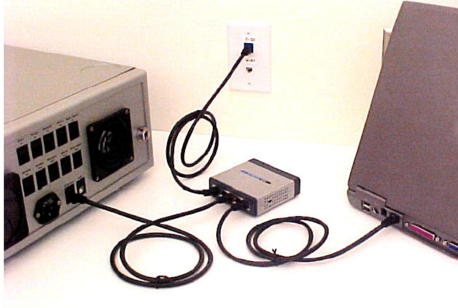
Figure D-9: Instrument and computer connected to LAN via Ethernet switch
