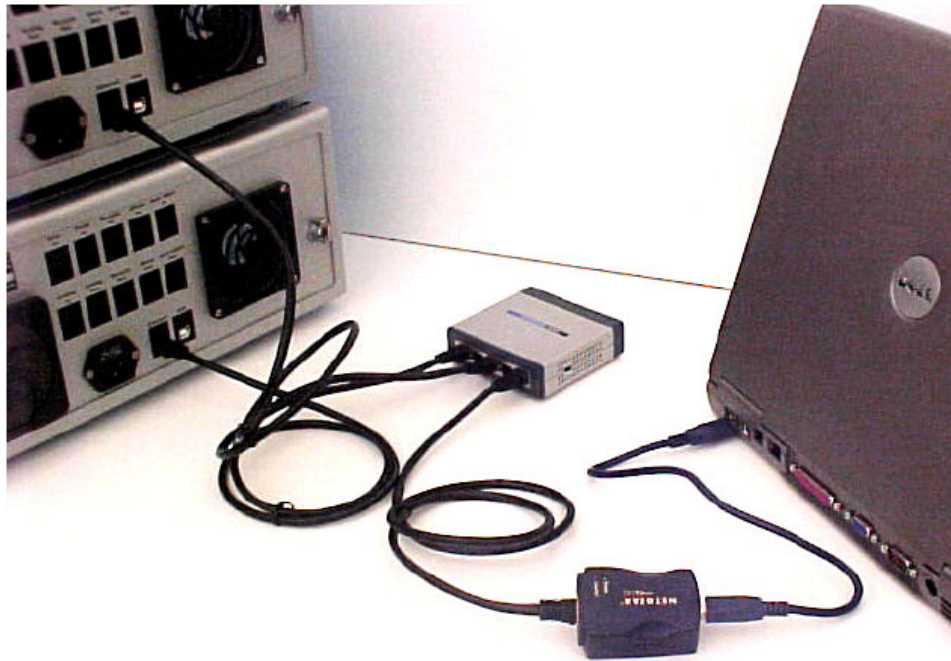
Figure D-14: Connecting two instruments to USB via Ethernet switch and adapter
