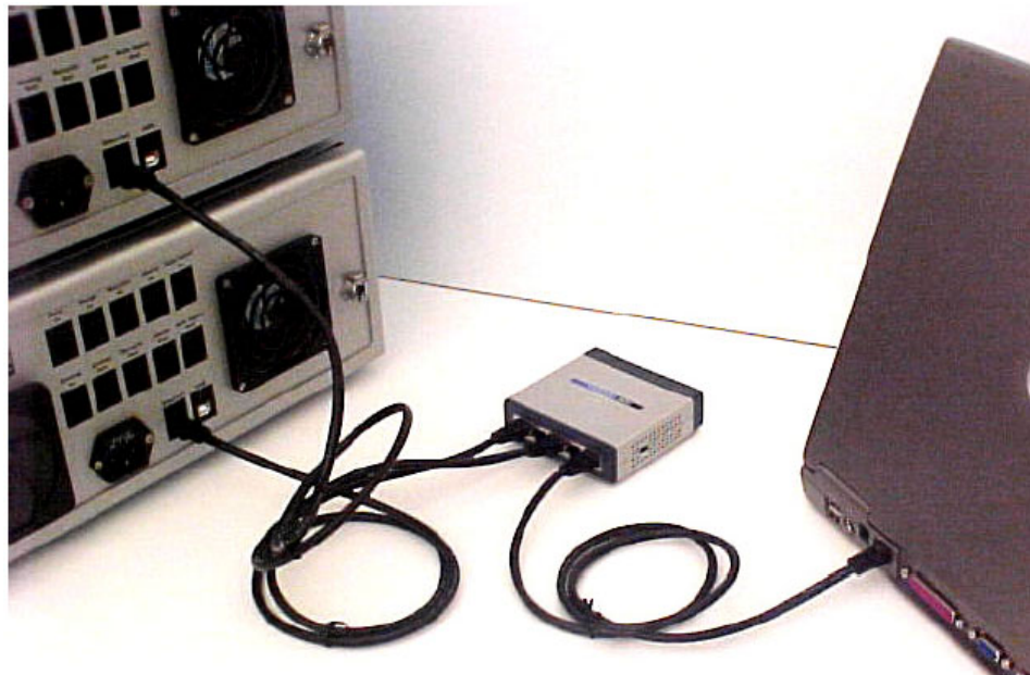
Figure D-17: Connecting multiple instruments to computer via Ethernet switch
