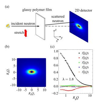
Figure S4. (a) Illustration of the SANS experiment on the uniaxially stretched polymers. (b) 2D SANS spectrum of the sample immediately after stretching to  $\lambda = 1.8$ . (c) Selected spherical harmonic expansion cofficients for the spectrum shown in panel b.
