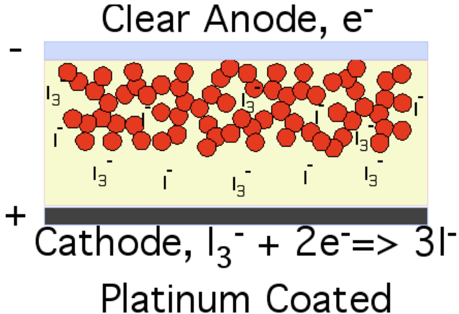
*Schematic of a Graetzel Cell. Red circles are titania aggregates coated with a dye. Pink background is an iodide electrolyte gel. Platinum coated cathode is at the bottom and a clear plastic sheet coated with fluorine doped tin oxide anode is at the top.*
