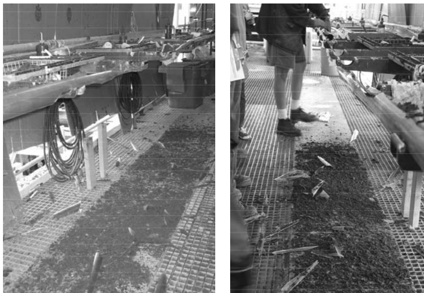
FIGURE 8.17 Core liner failures due to hydrate gas release on ship board.
