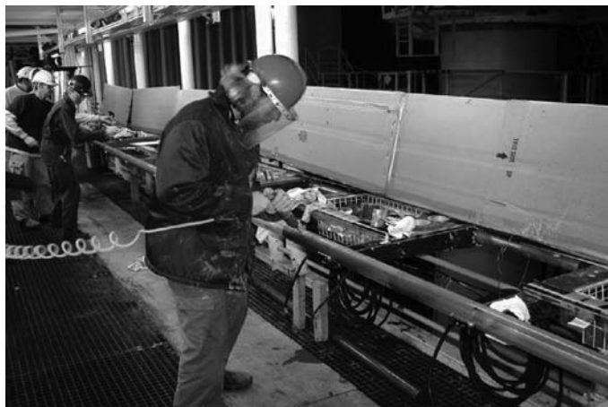
FIGURE 7.16 Shipboard drilling of gas pressure relief holes in hydrate nonpressurized core liner to accommodate gas hydrate dissociation. (Courtest F. Rack, May 5, 2004.)
