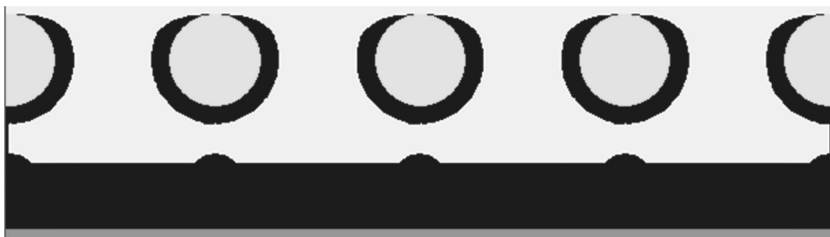
FIGURE 6.24. The liquid bridge snaps leaving a larger ink deposit directly beneath the mesh, and ~30% of the original ink wrapped around the mesh fiber.
