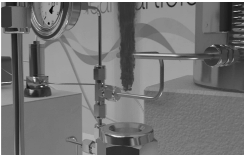
FIGURE 3.4. Production of iron oxide nanoparticles in a supercritical hydrothermal process.
