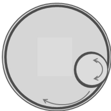
FIGURE 3.8. The ConCor™ grinding process.
