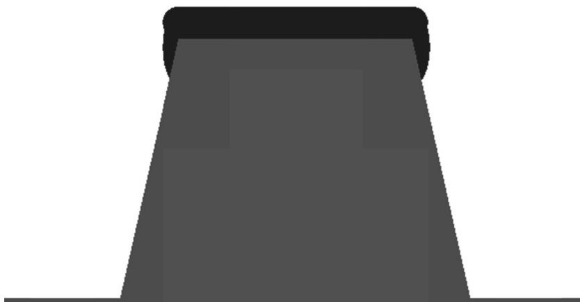
FIGURE 6.19. Ink accumulates along the edge of the dot, allowing, for example, ghost images outside straight lines.
