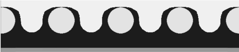
FIGURE 6.22. The squeegee is far away, allowing the mesh to come out of the ink—bringing some ink with it.
