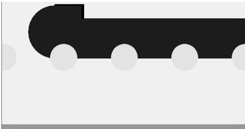
FIGURE 6.20. The flood bar partially fills the screen print mesh.
