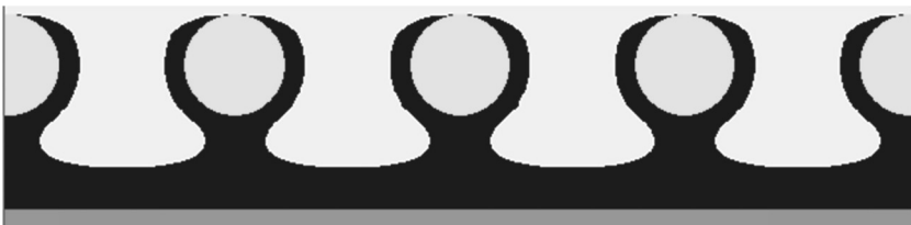
FIGURE 6.23. The ink naturally forms these menisci and liquid bridges.
