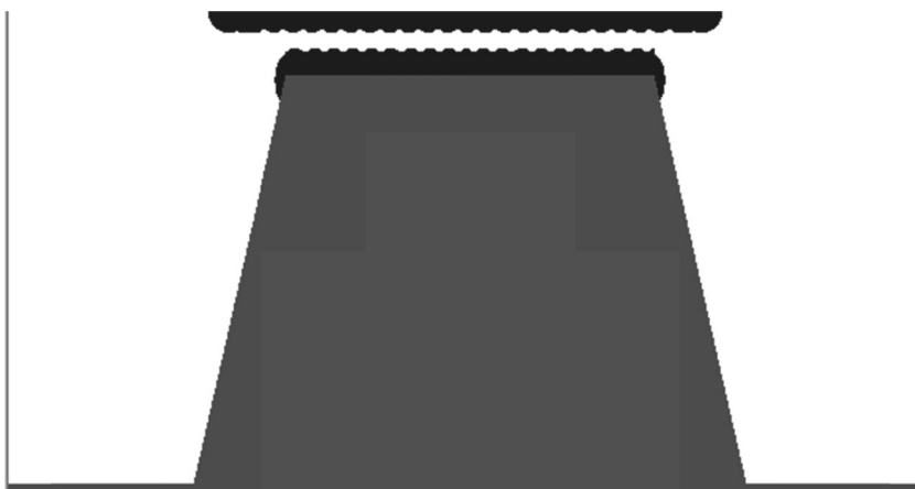
FIGURE 6.18. On separation, the coated dot is uneven because of the remnants of the voids.
