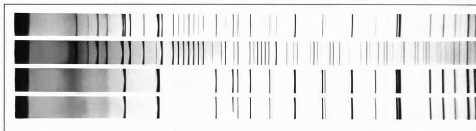
Figure 17 Single film with four powder patterns, made with Guinier-de Wolff camera. The two bottom patterns are of quartz, the third from the bottom is of ammonium alum, and the top one is of a mixture of quartz and ammonium alum. The range of 2\theta angles is 4^\circ to 82^\circ . (Courtesy of Enraf-Nonius Inc., Delft.)
