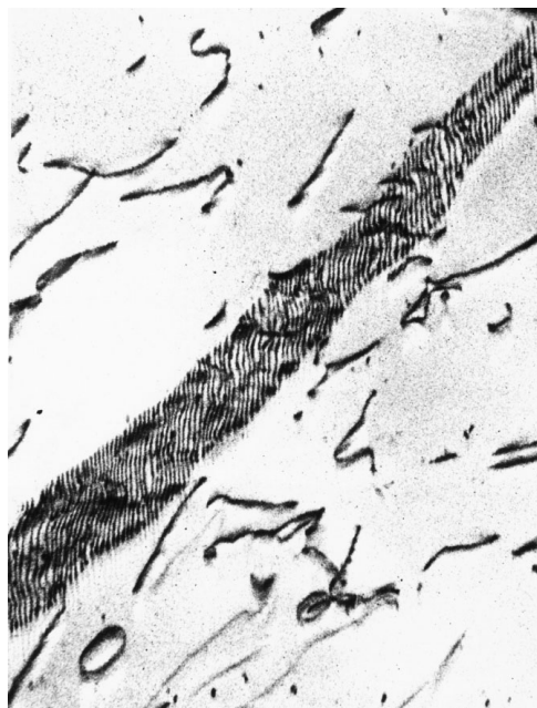
Figure 16 Lang topograph of a thin crystal of lithium fluoride. Dark lines are dislocations, some randomly arranged and some nearly parallel. The latter form the band running diagonally across the photograph; these dislocations, which intersect the top and bottom surfaces of the crystal, constitute a small angle boundary between two subgrains. of Mo K\alpha_1 radiation, 200 reflection. (Courtesy of A. R. Lang [21].)
