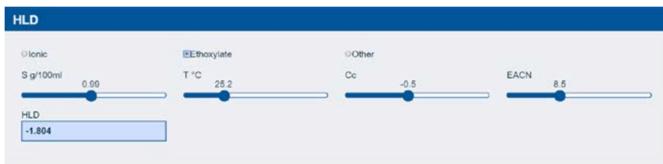
Figure 2-2 Back at room temperature the HLD is negative – this is an O/W emulsion
