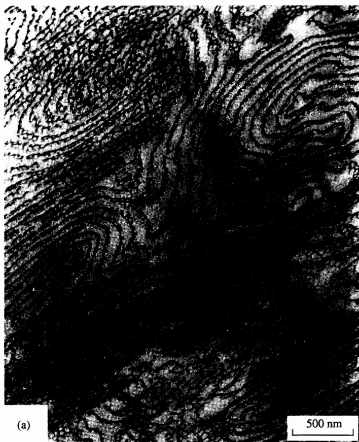
Fig. 2.35 Transition from folded lace to 'worm-like micelle' morphology in an f_{\text{PS}} = 0.81 \text{I}_2\text{S} copolymer (Pochan et al. 1996a). (a) TEM image of 'folded-lace' structure, following annealing of the sample at 120^\circ\text{C} for 1 week ( \text{OsO}_4 was used to selectively stain the PI); (b) 'randomly oriented worm' structure after annealing at 125^\circ\text{C} for 20 days; (c) Schematic of the transition from lamellae via 'folded-lace' to worm-like micelles.
