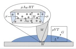
**FIG. 2**. Illustration of a system confined between the tip of an atomic force microscope and a substrate, as in the experiments of Ref. 5. From the thermodynamic point of view, it forms an open system confined in a slit pore with lateral area  $A_W$  and distance between walls H at a fixed temperature T and chemical potential  $\mu$  set by the liquid–gas equilibrium in the reservoir.
