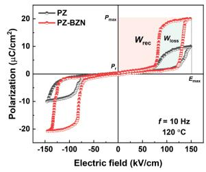
Fig. 3 Polarization - electric field double hysteresis loops of the PZ and PZ-BZN single crystals measured at 120 °C.
