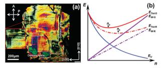
Fig. 5 (a) Domain structure of the (001)<sub>PC</sub> PZ-BZN single crystal observed under PLM at 220 °C. (b) Schematic diagram of the total energy ( $E_{Tot}$ ) as a function of the number of domain walls (n).  $E_V$  mainly represents the elastic energy in the crystal. O and R in the subscripts stand for the orthorhombic and rhombohedral phases, respectively
