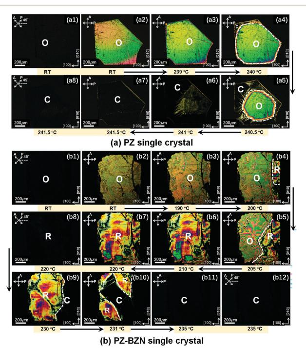
Fig. 4 Optical domain images of the  $(001)_{PC}$ -cut PZ (a) and PZ-BZN (b) single crystals under polarized light microscopy (PLM) with cross-polarizers at various temperatures (from room temperature to  $\sim$ 240 °C). O, R and C stand for orthorhombic, rhombohedral and cubic phases, respectively.
