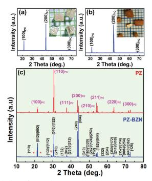
Fig. 1 (a and b) X-ray diffraction patterns of the naturally grown largest face of the PZ (a) and PZ-BZN (b) single crystals. The insets in (a and b) show the as-grown PZ and PZ-BZN single crystals, respectively. (c) XRD patterns of the PZ and PZ-BZN powders obtained from ground single crystals. The XRD patterns in (c) are indexed with both the pseudocubic setting (with subscript "PC") and the orthorhombic setting. The impurity peaks are marked by stars (\*).
