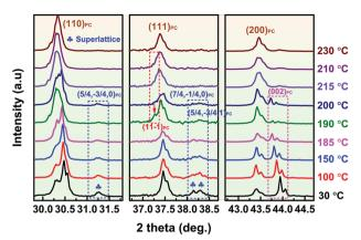
Fig. 6 XRD patterns of the ground PZ-BZN single crystals measured at various temperatures between 30 and 230  $^{\circ}$ C.
