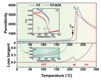
Fig. 2 Temperature dependences of the dielectric permittivity and loss tangent of (001)<sub>PC</sub>-oriented PZ and PZ-BZN single crystals measured at 100 kHz upon heating. The inset (1) shows the temperature dependence of  $1/\varepsilon_{r_{\ell}}$  which exhibits a linear relation above  $T_{C_{\ell}}$  following the Curie-Weiss law. The blue area in the dielectric permittivity curves is enlarged in
