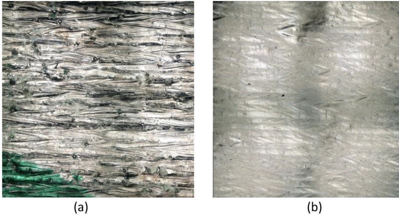
Fig. 13. Optical Microscopy image of 3 mm by 3 mm areas of SLM-AM samples used for the measurements - Rough (a) and Smooth (b).
