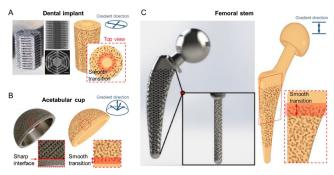
Figure 8. CNN-enabled generation of large gradient spinodal structures for fabricating various porous orthopedic implants: (A) dental implant; (B) acetabular cup and (C) femoral stem of hip implant. Images of the real implants are adapted from  $^{46-45}$ .
