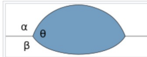
Figure 3: Coexistence of three fluid phases in mutual contact; here, \alpha , \beta , and \theta each indicate both a phase and its contact angle.
