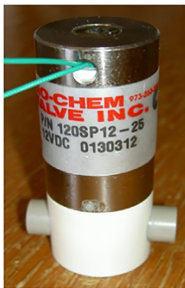
Fig. 25.24 Solenoid piston micropump.
