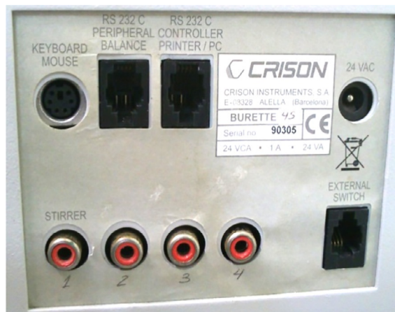
Fig. 25.19 Rear panel of the multisyringe burette.
