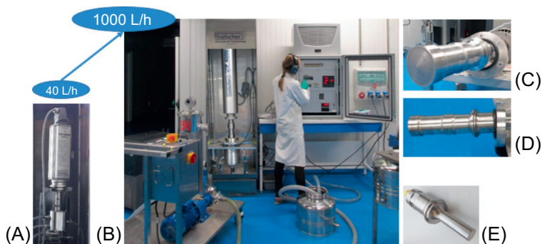
Fig. 12.4 Ultrasonic devices equipped with a probe: from lab to pilot scale. (A and E), lab scale probe with US chamber of 200 mL, 40 L/h. (B, C, and D), pilot ultrasound equipment with a 1 L US chamber, 1000 L/h.
