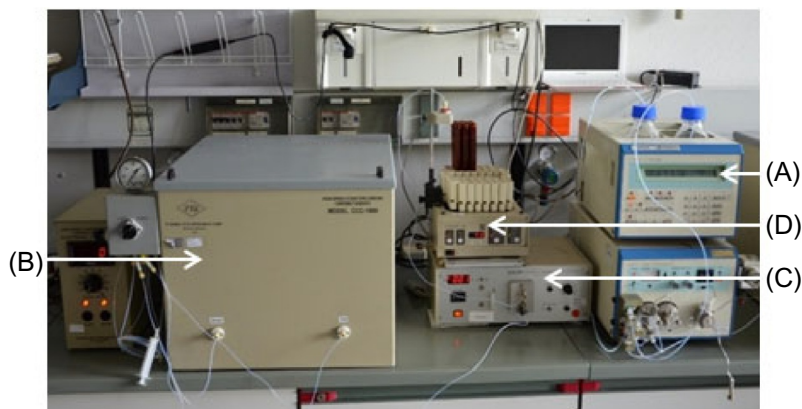
Fig. 10.5 Photo of the CCC-1000 setup with (A) pump; (B) CCC centrifuge; (C) UV/Vis detector; and (D) fraction collector. (Courtesy of M. Englert.)
