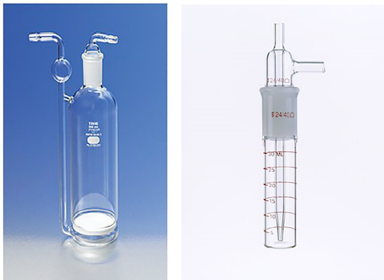
Fig. 1.5 Solvent extraction of gases using a bubbler ( left ) or impinger ( right ).
