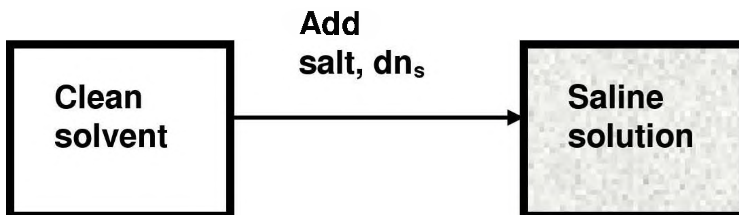
Figure 8.1. The constant volume cell in the Kirkwood-Buff charging process: Starting with a clean solvent, salt in small quantities is added to the container while maintaining a constant volume V^0 and constant temperature T^0 .
