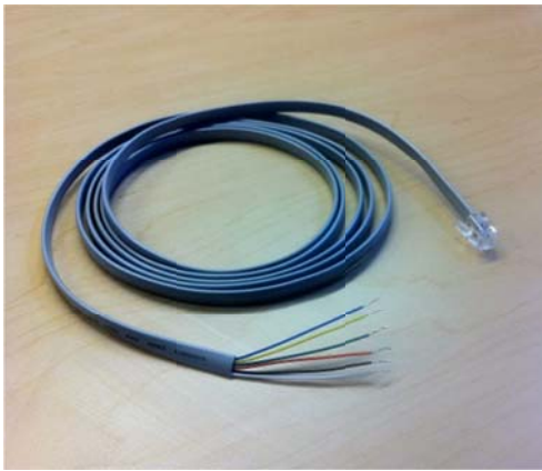
Fig. 11: HELEOS/TREOS RJ-12 cable p/n P4045-19
