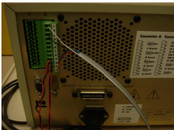
Fig. 5: Back Panel of Waters UV Detector
