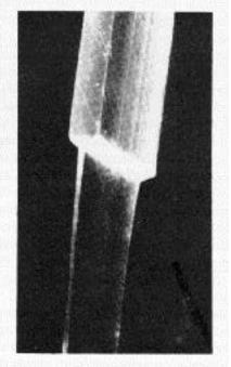
Figure 11.1. Photograph of a neck formed in the redrawing of oriented polyethylone.
