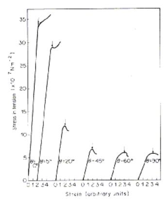
Figure 11.28. Stress strain curves for various angles # between the tensile axis and the initial draw direction for tensile tests on drawn polyethylene terephthalate sheets. The vield points are marked by arrows. [Redrawn with permission http://www.eng.uc.edu/~gbeaucag/ Classes/Characterization/
