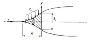
Figure 12.8. The Dugdale plastic zone model for a craze.
