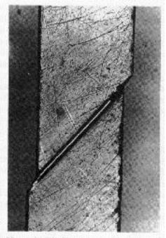
Figure 11.26. Photograph of a deformation band in an oriented sheet of polyethylene terephthalate.
