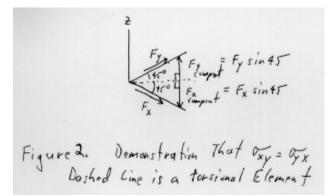
b) Assumptions: No rotational torque on the material.
