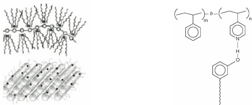
Figure -3 - Coordinated comb shaped polymeric supramolecules and their cylindrical self-assembly (left) 1 Structure of poly(styrene)- b -poly(4-vinylpyridine) (right) 1
