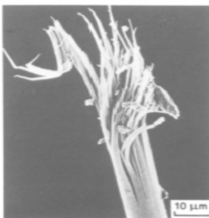
Fig 4: The fibrillar structure of a fractured Kevlar fiber 4
