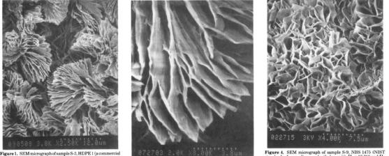
igure 1. SEM micrograph of sample S-3, HDPE 1 (a commercial igh density polyethylene with  $\dot{M}_n = 7300$  and  $\dot{M}_w = 43000$ ) rapid (coline).
