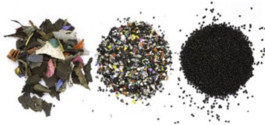
Fig. 3.14 Example of plastics before, during and after mechanical recycling, used with kind permission from MBA Polymers Austria GmbH. All rights reserved
