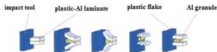
Fig. 6.6 Delamination process in a fractionator machine [14]
