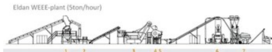
Fig. 8.7 Example of a setup of large WEEE recycling system ( 5 \text{ t h}^{-1} ) [7]. (1) Shredder. (2) Eddy current separator. (3) Tumble back feeder. (4) Multipurpose rasper. (5) Eddy current separator. (6) Heavy granulator. (7) Separation table
