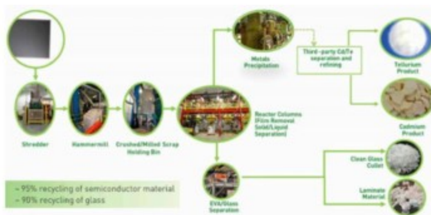
Fig. 11.5 PV cell recovery flowsheet
