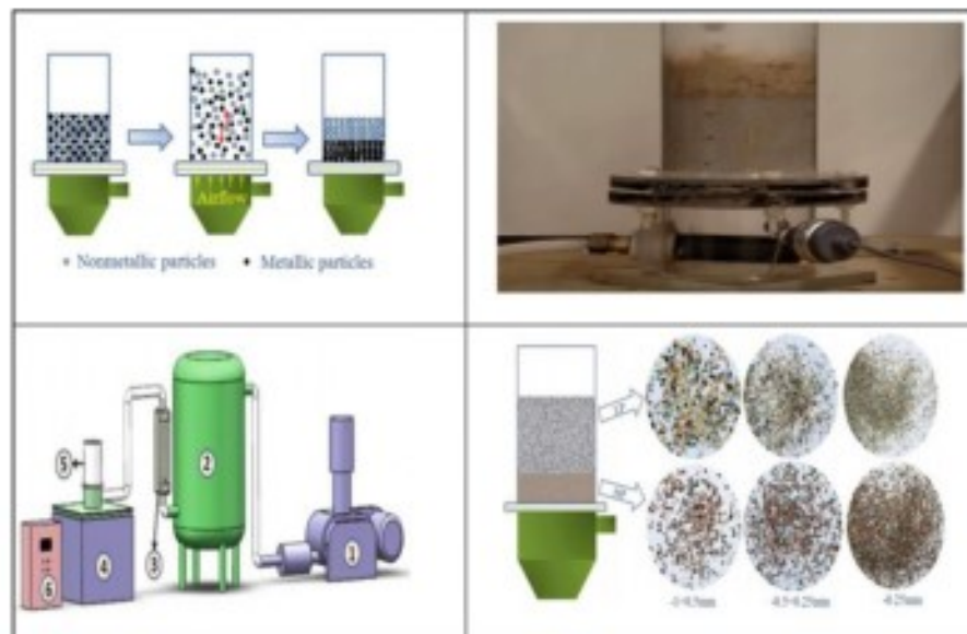
Fig. 7.12 Segregation process of metallic and nonmetallic particles in a vibrated gas-solid fluidized bed separation system: ① roots blower, ② 19 pressure tank, ③ rotameter, ④ vibrating table, ⑤ gas-solid fluidized vessel, ⑥ control unit. (Compiled from [23])
