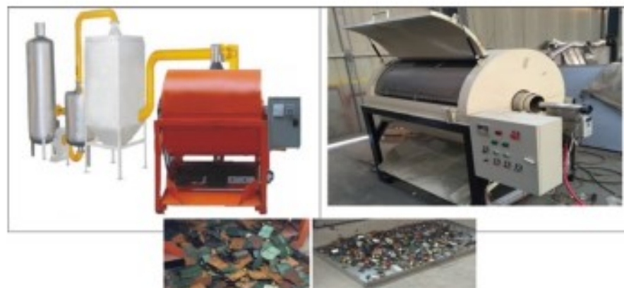
Fig. 4.3 Drum-type dismantling machine with air cleaning system and dismantled WPCBs and ECs developed in China
