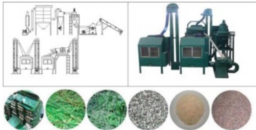
Fig. 7.21 PCB recycling flowsheet with ECSs, industrial equipment pictures, and feed products obtained
