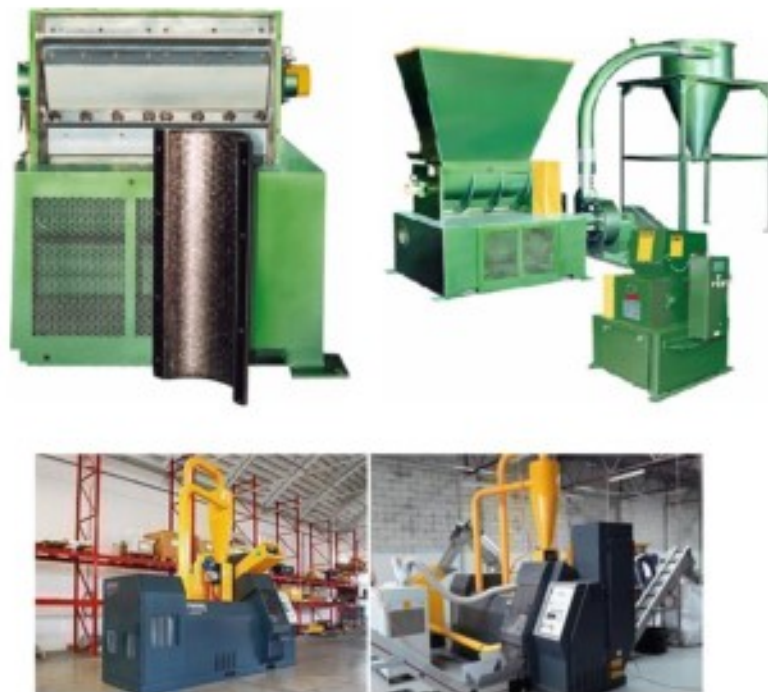
Fig. 6.5 Two different industrial-scale pulverizer machines along with screens and dust collection cyclones
