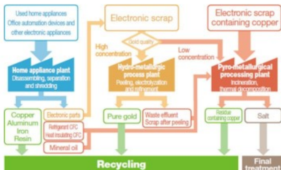
Fig. 8.11 DOWA's first e-waste hydro- and pyrometallurgical recycling plant flowsheet in China [13]
