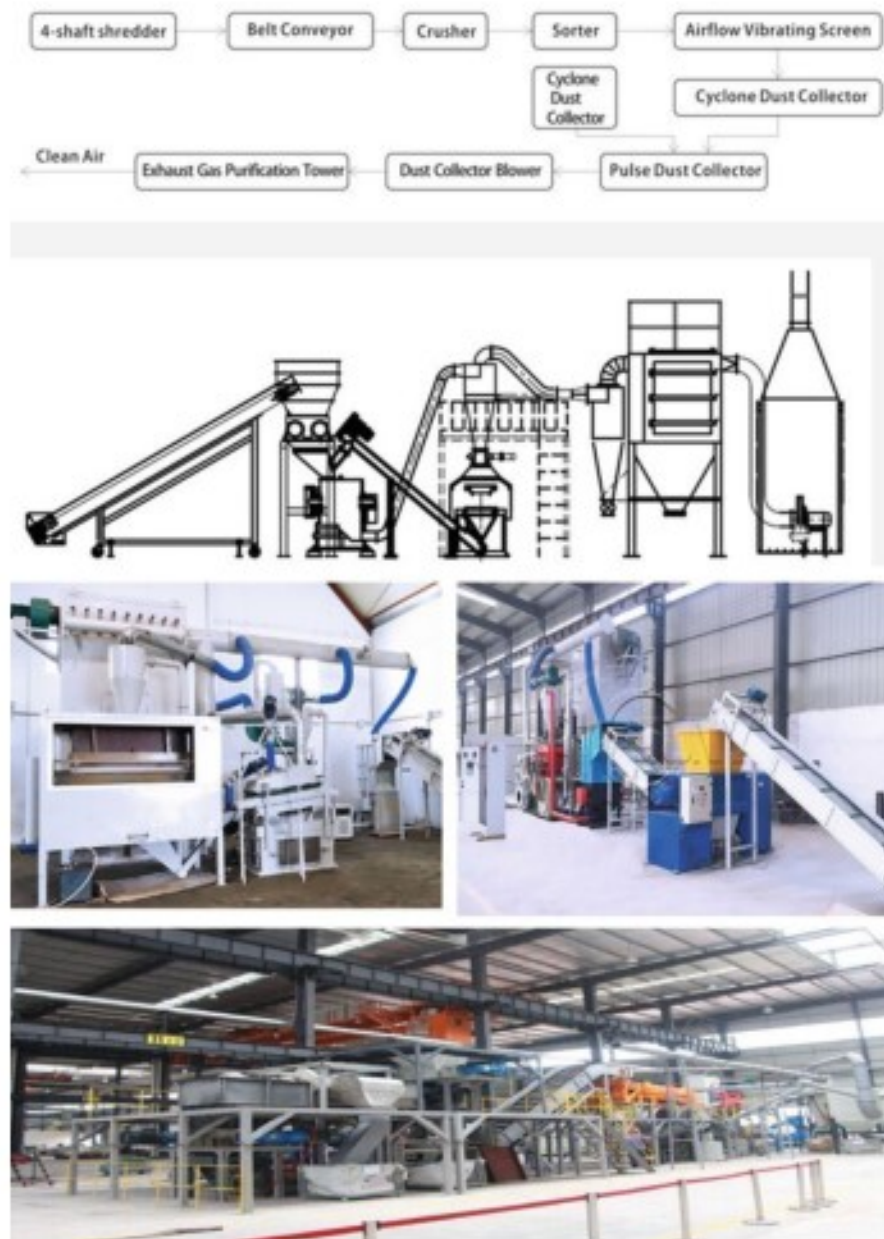
Fig. 8.3 Typical WPCB recycling flowsheet, layout, and industrial application pictures [3]
