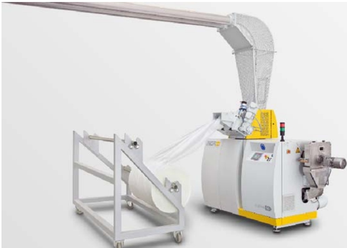
Figure 5.6 E:GRAN chopper–feeder–extruder combination. Sample stand-alone application: Feeding defective film via a roll feeder. Courtesy of Next Generation Recyclingmaschinen GmbH. NGR, Plastic recycling technologies. E:GRAN. https://www.ngr-world.com/product/egran/ .
