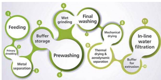
Figure 8.25 Schematic diagram of the Sorema film recycling process [19]. 1, Feeding; 2, Primary shredding; 3, Metal separation; 4, Buffer storage; 5, Prewashing; 6, Wet grinding; 7, Final washing; 8, Mechanical drying; 9, Thermal drying and aerodynamic separation; 10, Buffer for extrusion; and 11, In-line water filtration. Courtesy of Sorema.
