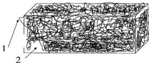
Figure 8.29 Asphalt pavement formed from an asphalt matrix (2) reinforced by fragments of flexible multilayer and/or monolayer plastic packaging (1) (2010, BRPI0804756 A2, COSMO ANTONIO EUFRASIO DE ARAUJO).
