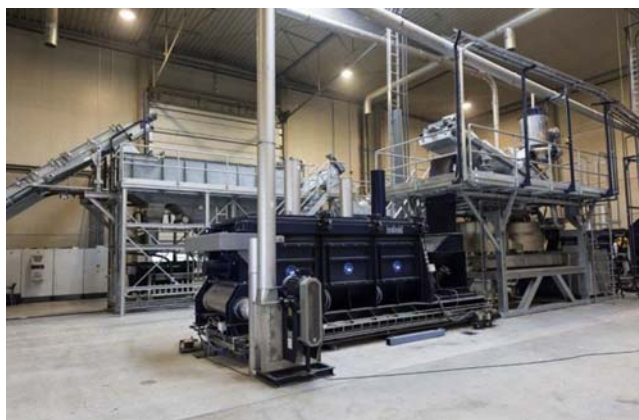
Figure 8.19 Hydrocyclone and dryer, in the background a prewashing unit [16]. Courtesy of Herbold Meckesheim GmbH.
