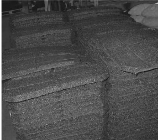
Figure 7.4: Moulded barrier products have been manufactured using rubber crumb and shred from used truck tyres. Reproduced with permission from the WRAP Quality Protocol, Waste and Resources Action Programme, Banbury, UK. ©WRAP (see note with Figure 7.1 ). appearance, steel or coloured rubber inlays can be added at the moulding stage. A number of products can be successfully manufactured by ILP in this way, including sound and vibration dampeners, rubber mats, rubber transportation wedges, and steel-reinforced rubber traffic posts.
