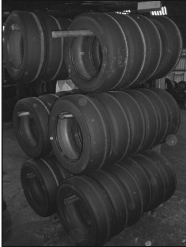
Figure 5.1: Passenger tyre carcasses retreaded with compounds containing 5–30% DevulCO 2 rubber prior to moulding. Reproduced with permission from the DevulCO 2 Research Project Consortium (Lead Partner: Smithers Rapra, Shawbury, UK), UK. ©2012, DevulCO 2 .
