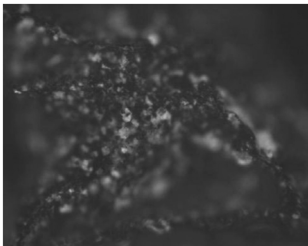
Figure 4.8: Fine rubber particles suspended in water and aerobically treated with desulfurising bacteria – WRAP DART project. Reproduced with permission from WRAP, Banbury, UK.
