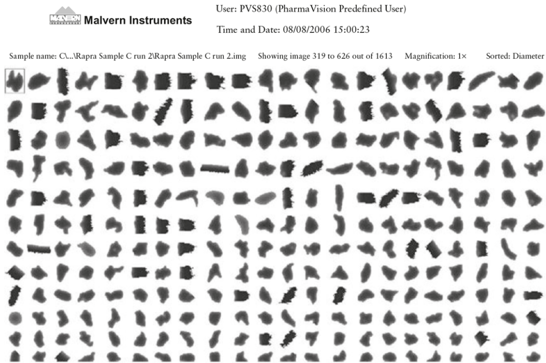
Figure 6.10: Profile images generated using a particle analyser of rubber crumb produced using a water jet process. Reproduced with permission from Smithers Rapra Technology Ltd, Shawbury, UK.
