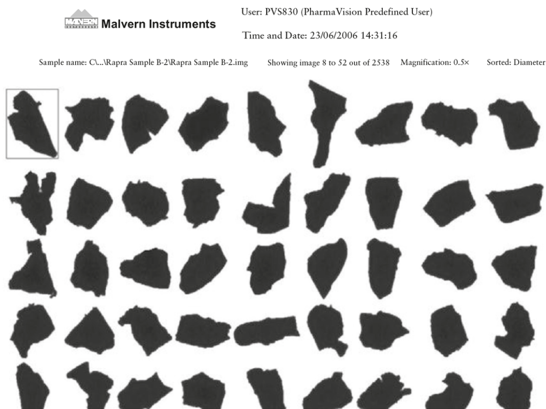
Figure 6.9: Profile images generated using a particle analyser of rubber crumb produced using a cryogenic process. Reproduced with permission from Smithers Rapra Technology Ltd, Shawbury, UK. ©2006, Smithers Rapra Technology Ltd.
