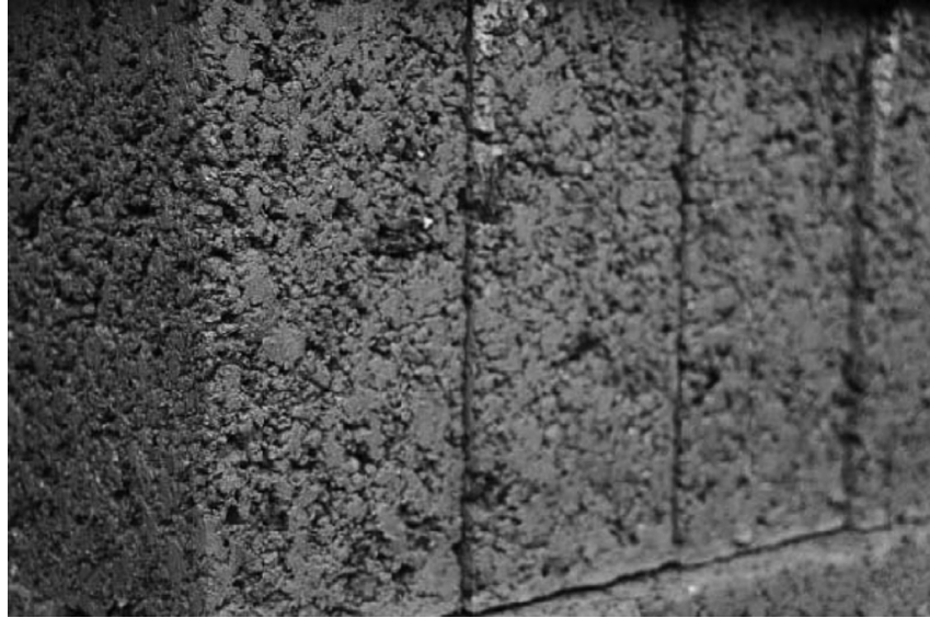
Figure 7.1: Lightweight construction blocks for the construction industry manufactured using waste tyre rubber as a partial replacement for aggregate. Reproduced with permission from the WRAP Quality Protocol, Waste and Resources Action Programme (WRAP), Banbury, UK. ©WRAP. Note: WRAP does not warrant that the functions contained in the material contained in this Site will be uninterrupted or error free, that defects will be corrected, or that this Site or the server that makes it available are free of viruses or bugs or represents the full functionality, accuracy, and reliability of the materials.
